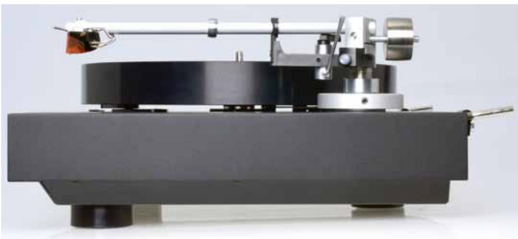
Barely visible from the side: owing to the subchassis, the platter bearing and arm base hover slightly above the surface of the PE chassis. Yet clearly recognisable from the side: the high-built 3 kg (6.6 lbs) aluminium platter and the upmarket TP92 tonearm from Thorens.
