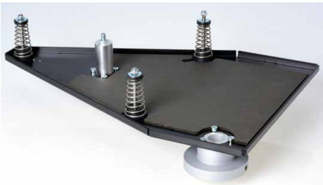
The heavy aluminium subchassis is lavishly dampened. The three conical springs are fitted with guide bolts against nutation and tensioned unevenly, as they are not centrally loaded. Above centre the platter bearing, the screw serves to fine-tune the weight uptake between ball and magnet.
