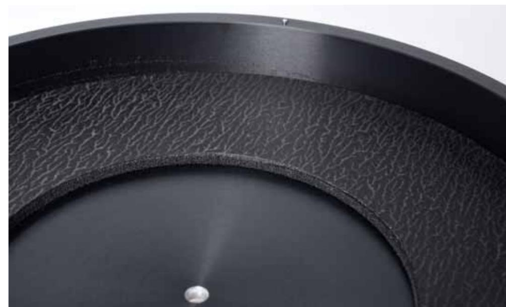
The heavy main platter of turned and anodised aluminium is generously dampened on the inside against vibrations and resonances: a layer of special foam soothes the surface, another layer of bitumen gives the damping sufficient mass and inertia.
